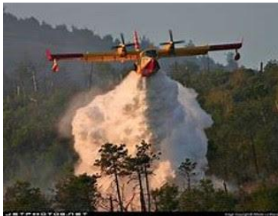
Figure 4: Canadair CL415 “Super Scooper”. Note ability to carry out low altitude drops, increasing effectiveness.
