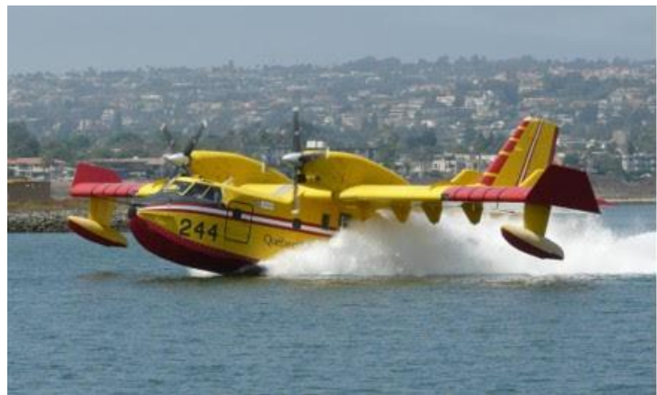
Figure 4: Canadair CL415 “Super Scooper”. Note ability to carry out low altitude drops, increasing effectiveness.
