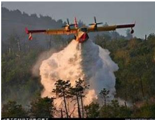
Figure 3: Canadair CL415 “Super Scooper”. Note ability to carry out low altitude drops, increasing effectiveness.
