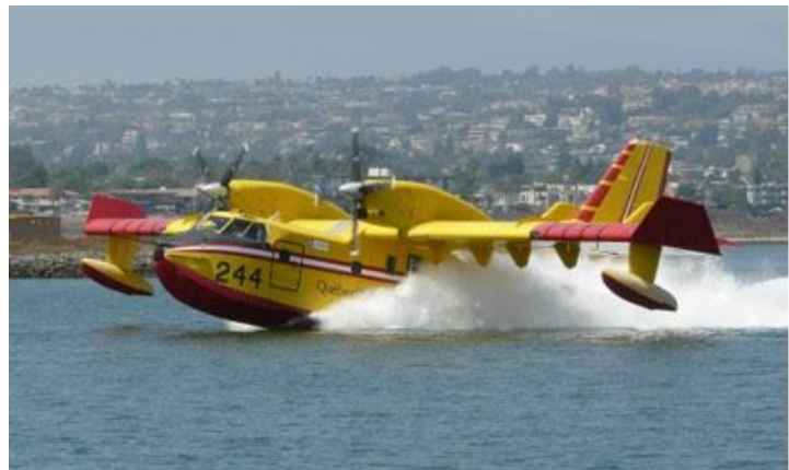
Figure 3: Canadair CL415 “Super Scooper”. Note ability to carry out low altitude drops, increasing effectiveness.
